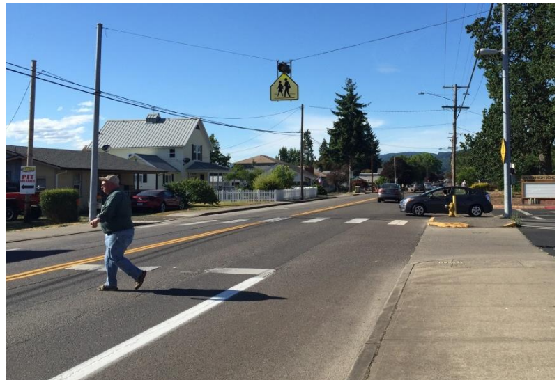
Overhead flashing pedestrian sign at the High School entrance along Main Street
