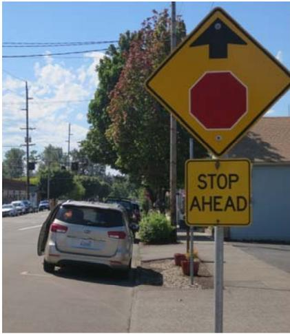
*This STOP AHEAD sign, located on Ridgeway east of Oatfield, should be on a separate signpost. The City should consider moving the STOP AHEAD sign closer to the STOP sign to which it applies, and replacing it with a Stop Ahead symbol sign.*
