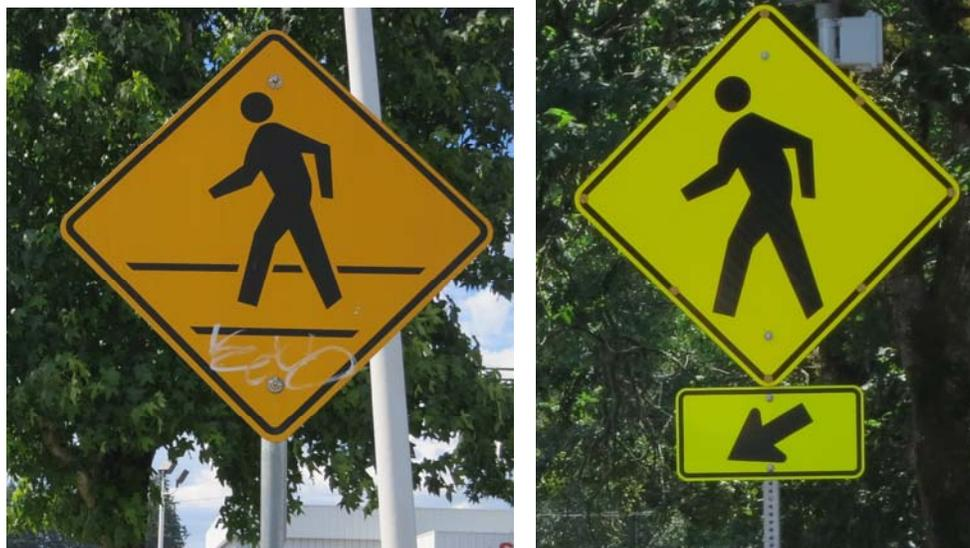
*The sign on the left, located on River Road at Gloucester, is the old-style sign with the crosswalk lines. The sign on the right is the new style with a diagonal arrow located at the crossing point.*
