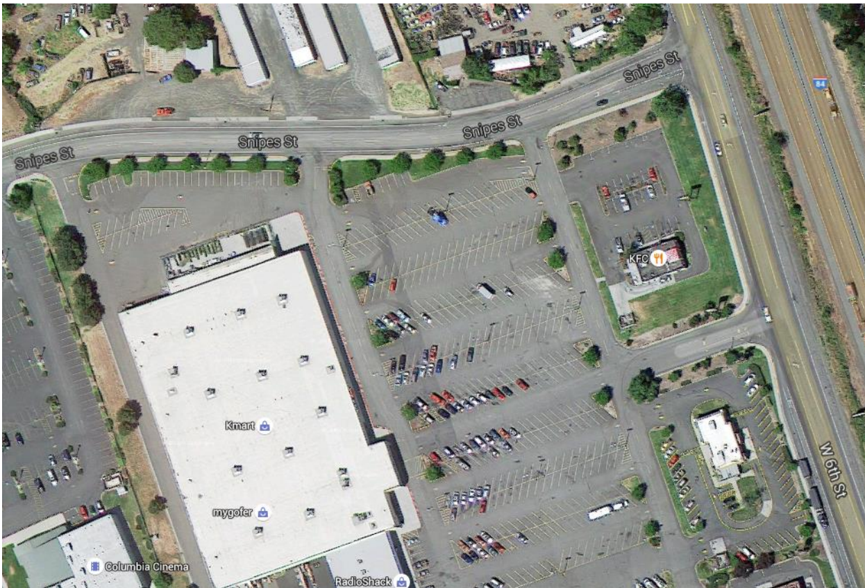
Exhibit 5-5: Example of Promoting Access on the Lowest-order Roadway Adjacent to a Parcel. (Source: Google Earth)
