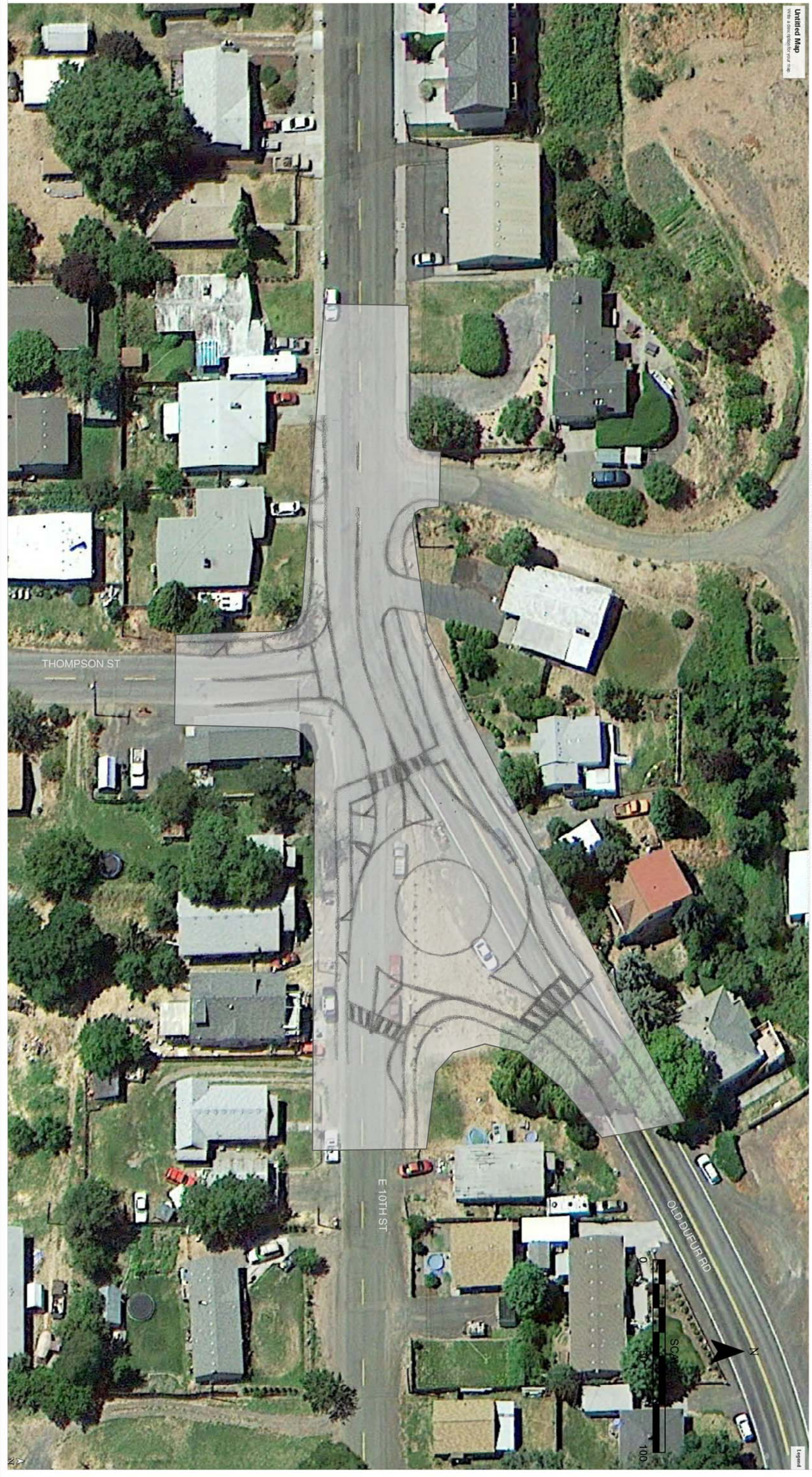
PROJECT I-6: CONCEPTUAL ROUNDABOUT & T-INTERSECTION THOMPSON ST/E 10TH ST/OLD DUFUR RD THE DALLES, OR
