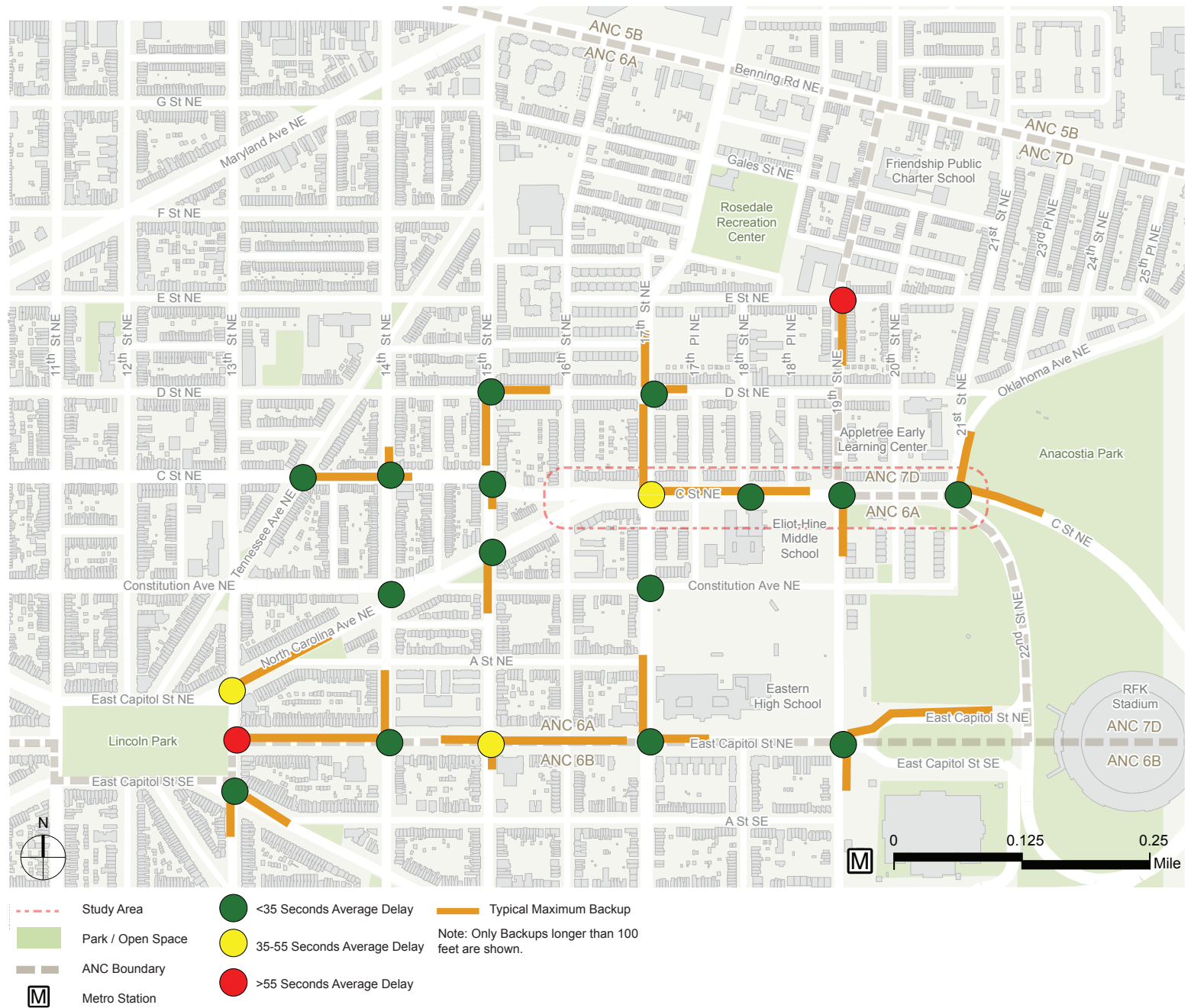
FIGURE 17. 2040 NO-BUILD TRAFFIC OPERATIONS (AM PEAK HOUR)
