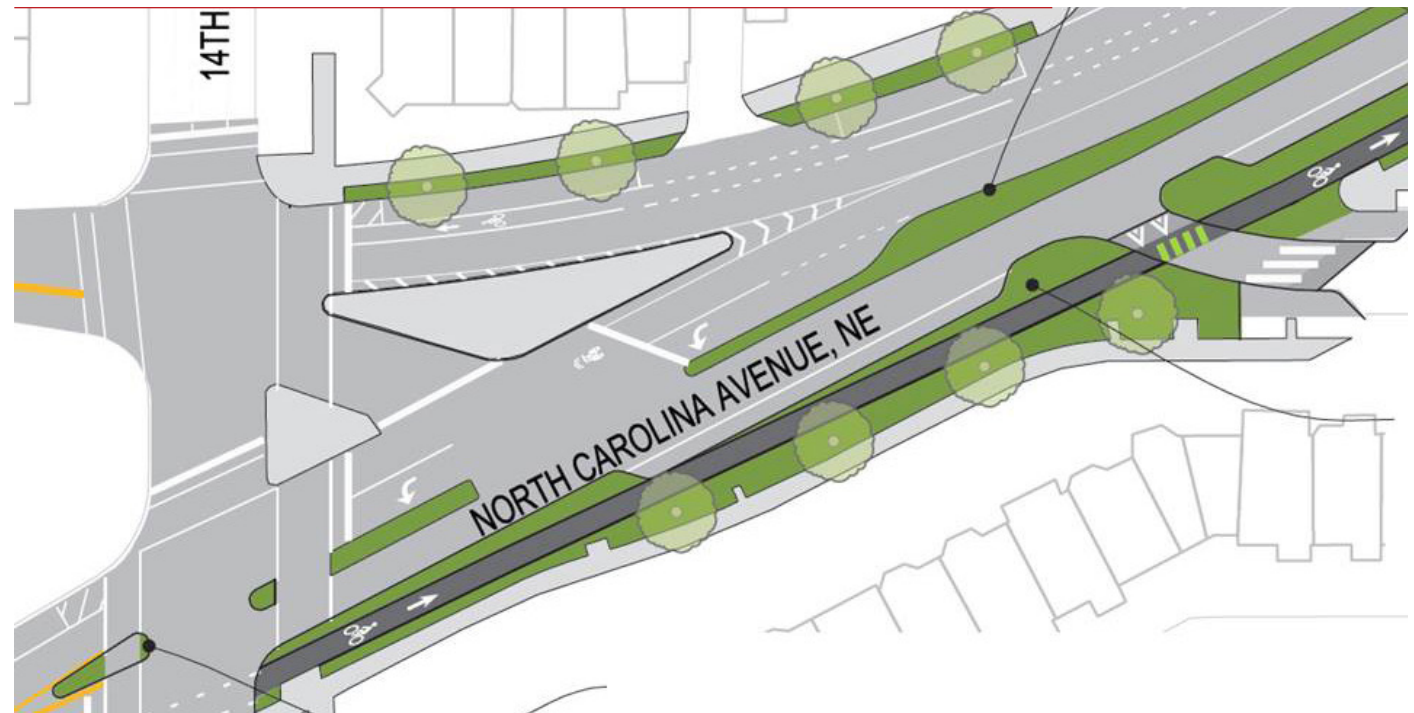
Recommended modifications at the North Carolina Avenue NE/Constitution Avenue NE/14th Street NE intersection.
