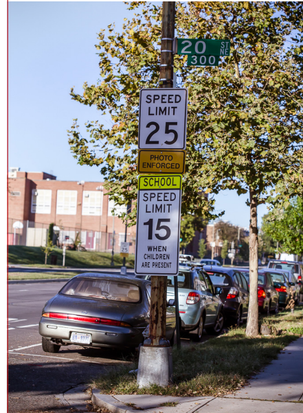
Posted speed limits on the study corridor. Measured speeds are well above both posted speeds.
