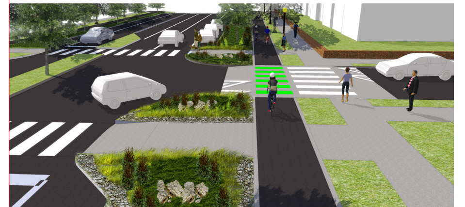
Raised crosswalk and bike crossing at 17th Street NE.
