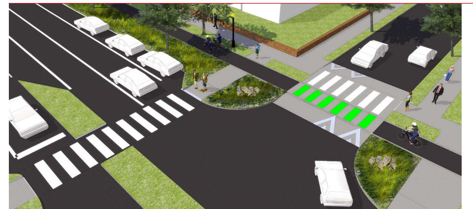
Raised crosswalk and bike crossing and curb extensions at 17th Street NE.
