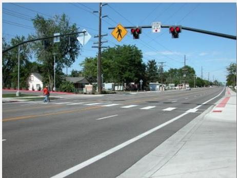
A HAWK is a pedestrian-activated signal that is unlit when not in use. When activated the signal begins with a yellow light alerting drivers to slow and then a solid red light appears requiring drivers to stop while pedestrians have the right-of-way to cross the street. HAWKs are often used on wide roadways where mid-block crossings are difficult.
