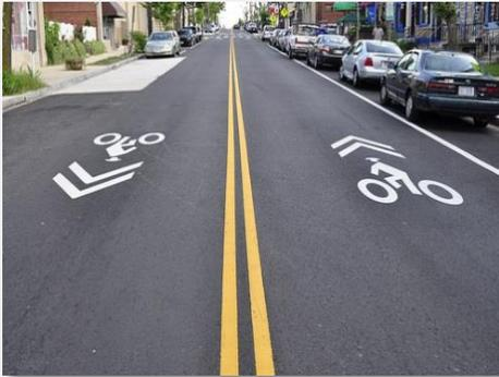
A shared-lane pavement marking, or sharrow, is a pavement marking that can be used where space does not allow for a bike lane and/or where vehicular volumes and travel speeds allow cyclists to comfortably and conveniently “share the road” with motorists. Sharrows remind motorists of the presence of bicycles and indicate to cyclists where to safely ride within the roadway.
