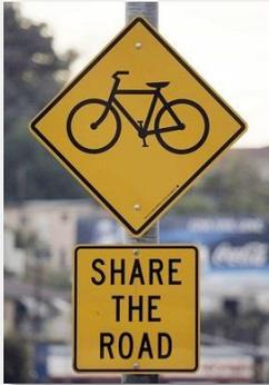
“Share the Road” signs can be used to remind drivers to watch for bicyclists on roadways without on-street bicycle lanes. However, the signs are not meant as a replacement for using the other facility types listed in this table. An alternative to the “Share the Road” sign is a “Bikes in Road” sign that suggests bicyclists take the lane rather than share the road.
