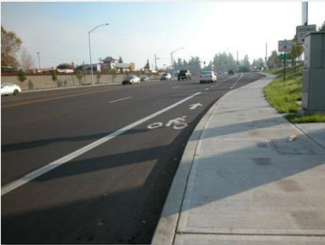
Bike lanes are on-street bicycle facilities that provide a designated space for cyclists that is separated from vehicle traffic by pavement markings. Bike lanes are generally used on collector and arterial streets with adequate space to accommodate the bike lane width and with vehicular travel volumes and speeds that make it difficult for drivers and cyclists to “share the road.” Bike lanes typically include white striping with a bicycle symbol or they can be buffered as shown below.
