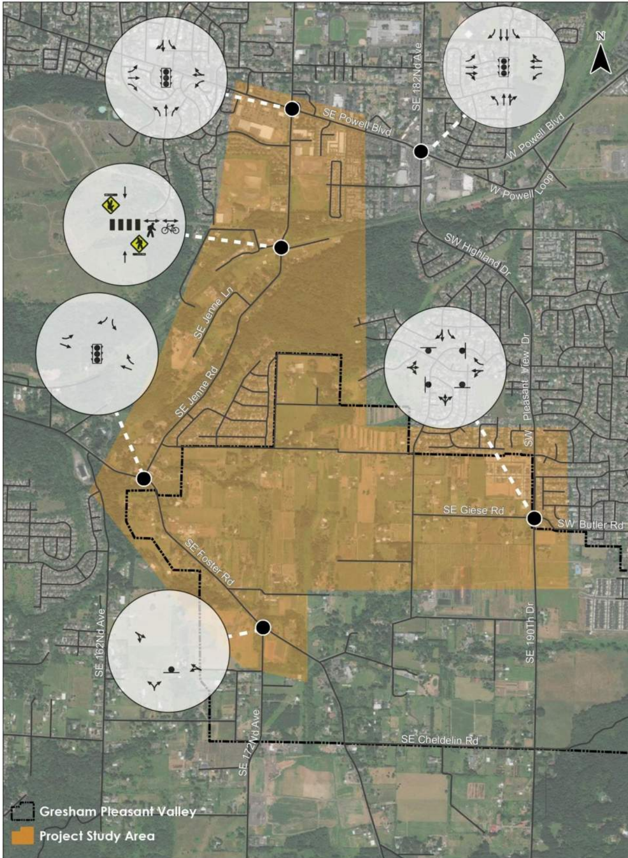
Figure 2 – Existing Lane Configurations
